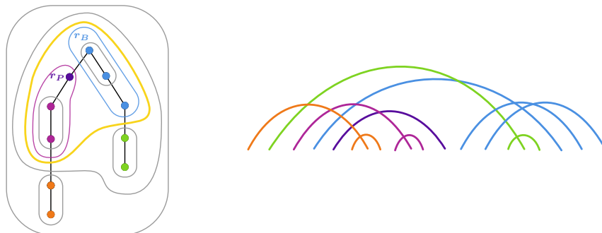
Figure 4.7: Example of a path tree partitioned with markings B, P, L , and R and its corresponding chord diagram.
